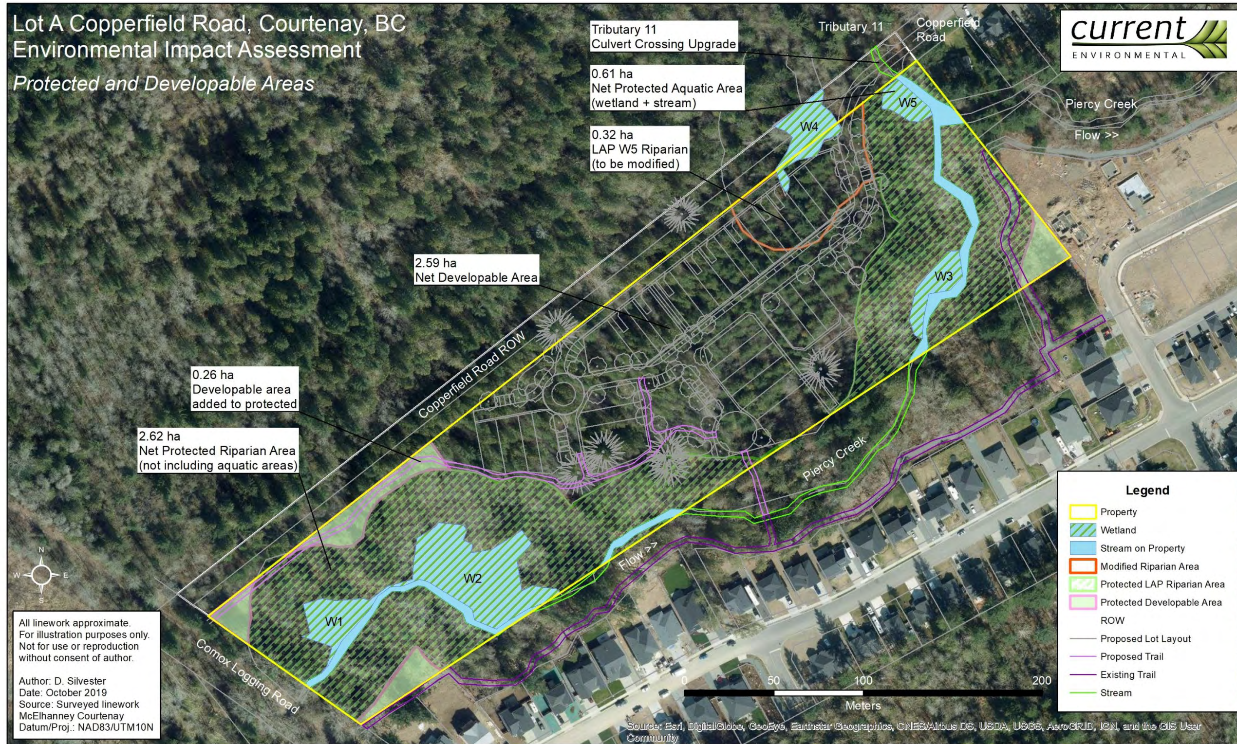
Figure 2. Site plan showing Environmentally Sensitive Areas (ESA) on the subject lot including wetland, riparian, and setback areas.
