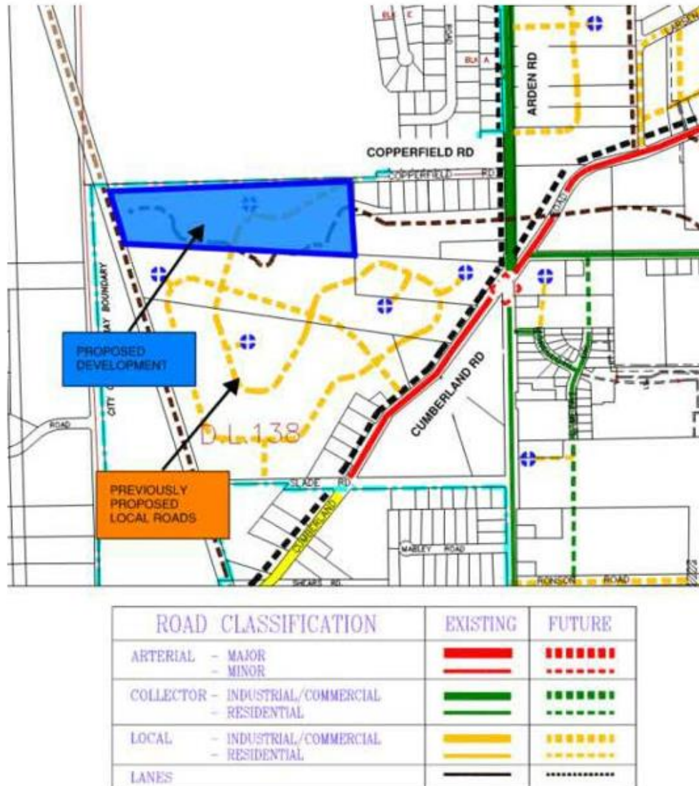
Figure 2: Future Road Network - City of Courtenay OCP Road Network Map No. 3 (2007) (Modified)
