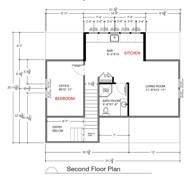
To meet the requirements for "no interior access to any part of the accessory building below the carriage house" as defined in the zoning bylaw, my application documents included the drawing below which shows the proposed location where we would erect a new internal wall. The space created by this wall would become the storage / laundry room for the suite above.
