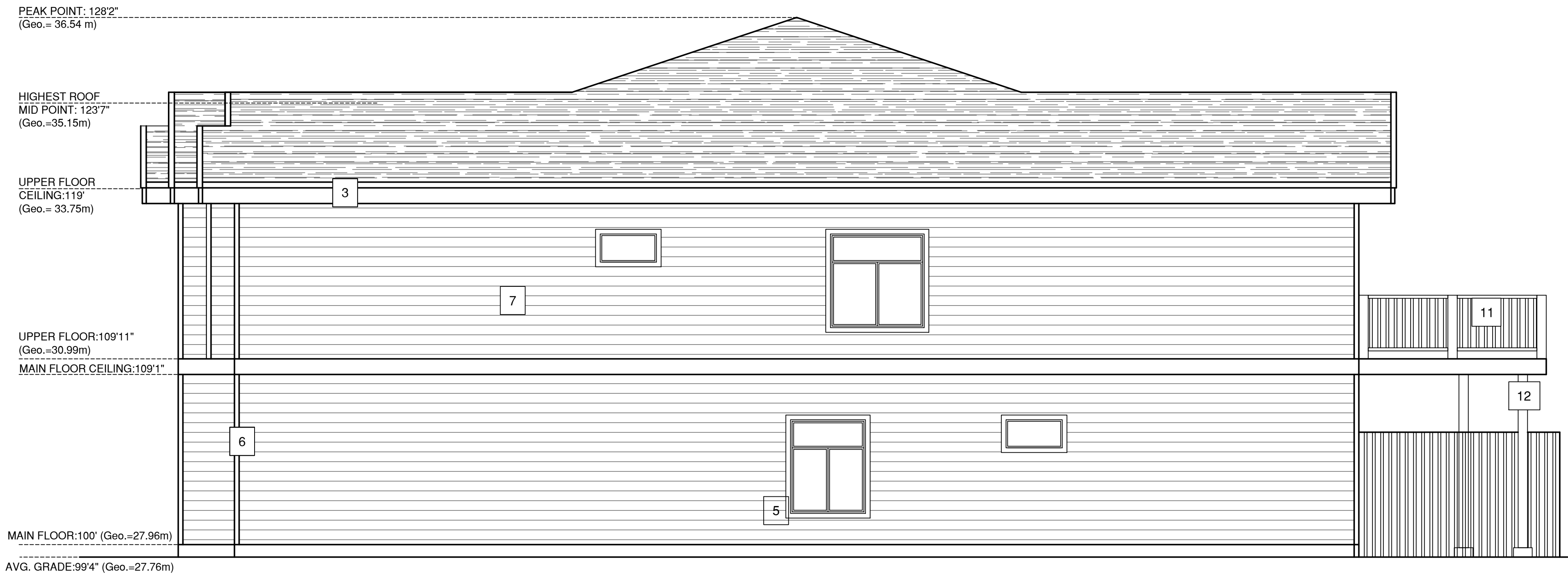
RIGHT SIDE ELEVATION SCALE: 1/4" = 1'-0"
